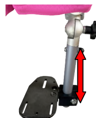
pic. 15: footplate height adjustment and other adjustments
